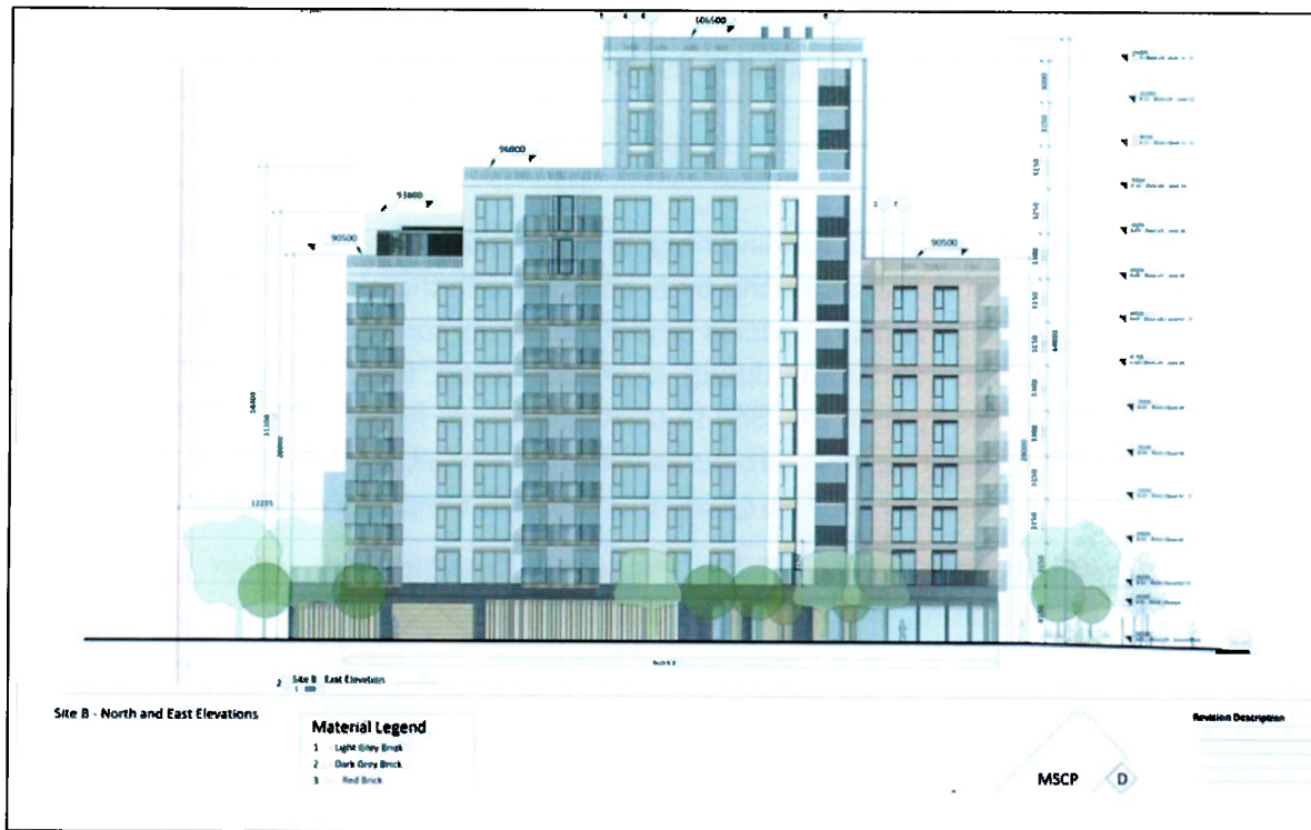
Figure 5-9: Example of the proposed building façades and heights, with opaque materials comprising coloured brick, panelling and metalwork throughout (Adapted from OMP drawing 20053-OMP-SB-XX-DR-A-2000 - Site B - North and East Elevations).
